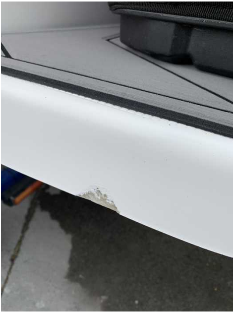
Starboard Hull defects, cracks, holes etc. Anchor drain vent squashed Scratches
